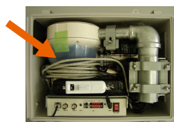
JPN Company F Portable Surveillance Camera System
