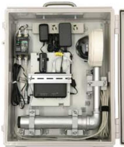
Carry the all-in-one trunk to the place to install the camera and plug the power. You can observe all around view from the remote place by your PC.
